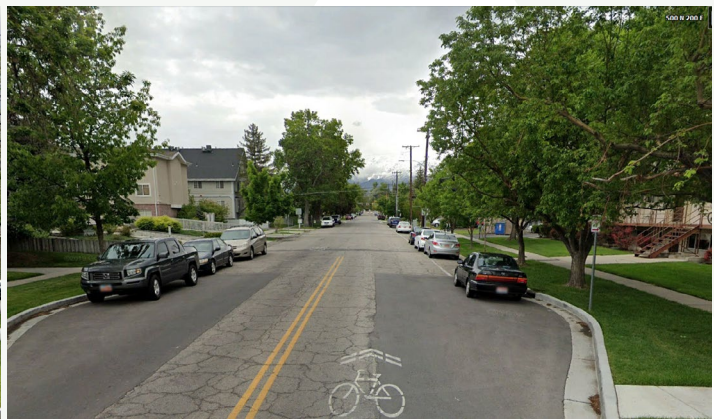
Street-level views of 200 E in Provo. Note that markings, bulb-outs, trees, and on-street parking visually narrow the roadway to decrease speed. The trees will also provide shade and reduce road noise for pedestrians.
