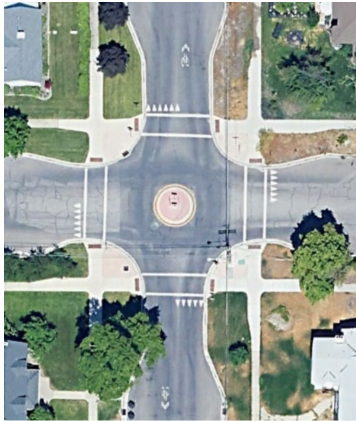
Mini traffic circles can manage vehicle speeds while improving flow for both vehicles and bicycles on local streets. The mountable curb allows emergency vehicles to proceed straight through, but the circle can also be landscaped for beauty and character (200 E and 200 N, Provo)
