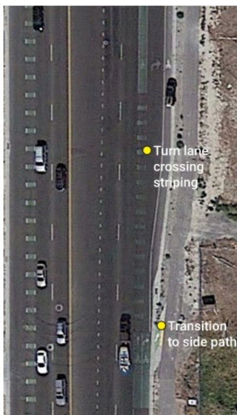
Right turn lane crossings and side-path transitions together provide options for cyclists (Redwood Road, Saratoga Springs)
