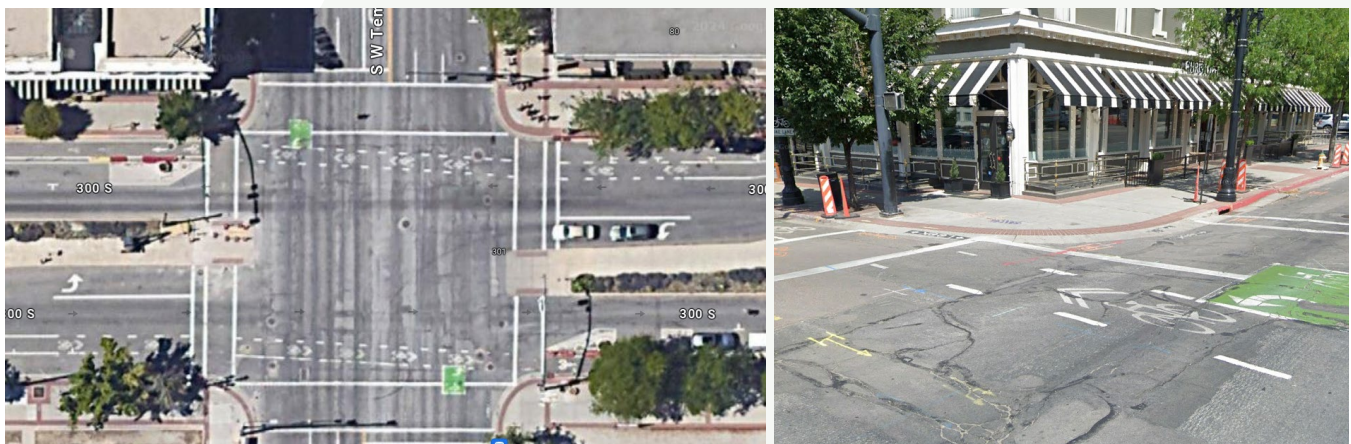
300 S W Temple in Salt Lake - Bike boxes and striping assisting with left turns from a protected bike lane.
