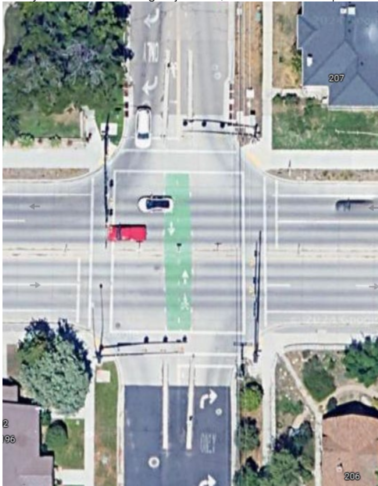
300 S and 200 E in Provo - Curbing protects bicycles approaching the intersection, prohibits crossing movements for vehicles, but allows active transportation users passage. Green pavement increases visibility for bicyclists.
