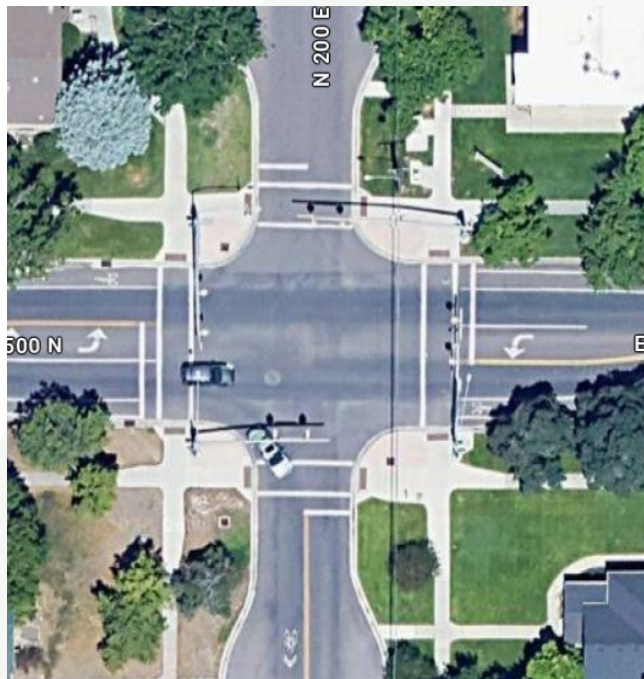
200 E 500 N Provo – Bulb-outs on the minor street with a sharrow calms traffic to make it a more comfortable bicycle facility.
