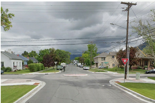
Street-level views of 200 E in Provo. Note that markings, bulb-outs, trees, and on-street parking visually narrow the roadway to decrease speed. The trees will also provide shade and reduce road noise for pedestrians.
