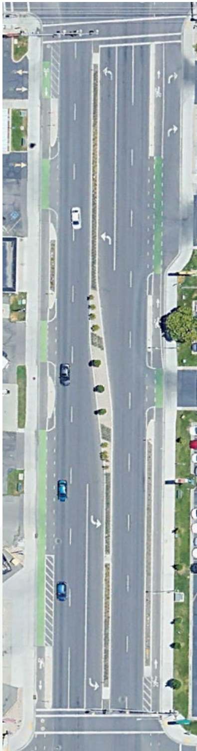
Painted driveway and right turn lane crossings remind drivers to look for bicyclists (Cougar Blvd, Provo)
